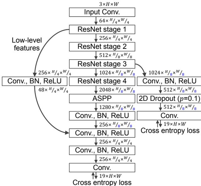
**Figure 2:** Detailed architecture of the baseline model
