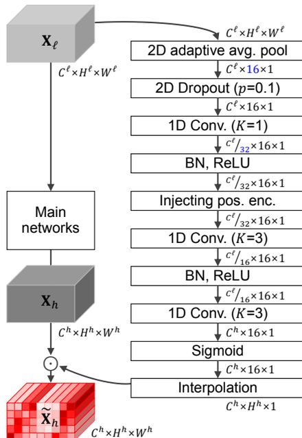
**Figure 1:** Detailed architecture of HANet.  $p$  denotes the dropout probability, and  $K$  denotes the kernel size of each one-dimensional convolution layer. BN denotes a batch normalization layer.
