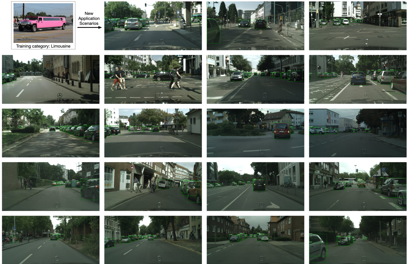
Figure 4. Qualitative results of our 5-shot car detection on Cityscapes. We visualize the bounding boxes with score larger than 0.8. The first image is a training example.
