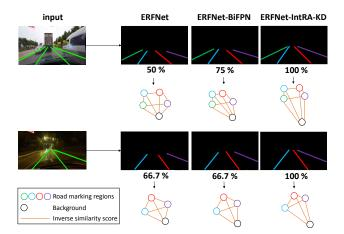
Figure 3: Visualization of the affinity graph generated by different methods. For visualization, we represent edges in an affinity graph by the inverse similarity score. The number below the segmentation map is  $F_1$ -measure.
