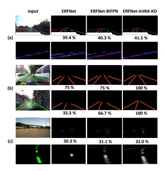
Figure 2: Qualitative results of different algorithms on (a) ApolloScape, (b) CULane and (c) LLAMAS testing sets. The number below each image denotes the accuracy for (a) and (c),  $F_1$ -measure for (b). Ground-truth labels are drawn on the input image. The second row of (a) and (c) are the enlarged areas covered by the red dashed rectangle.
