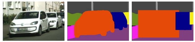
Figure S1: Weak Supervision Left: input image; Middle: fully supervised pixel association; Right: Weakly supervised pixel association. In this example, orange, blue and yellow color indicates the pixels which are assigned to a bounding box target of the three cars during training.
