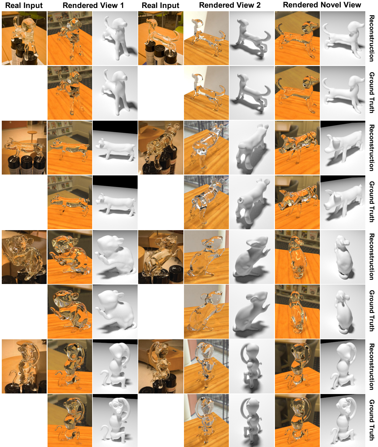
Figure 1. Results on 3D reconstruction for four real transparent objects. All shapes are reconstructed from 10 views, except the monkey in the last row that uses 12 views. We first present reconstruction results from two input views (columns 1-6). From left to right, the odd rows show the input image and the reconstructed shapes under different lighting and materials. The corresponding outputs using the ground-truth shapes rendered from the same view are shown in the even rows. We also render the reconstructed shapes and ground-truth shapes from a novel view direction that has not been used to build the visual hull (columns 7-8). In each instance, we observe that the reconstructions are close to the ground truth despite the challenging shapes, complex light paths and small number of views used for 3D reconstruction.
