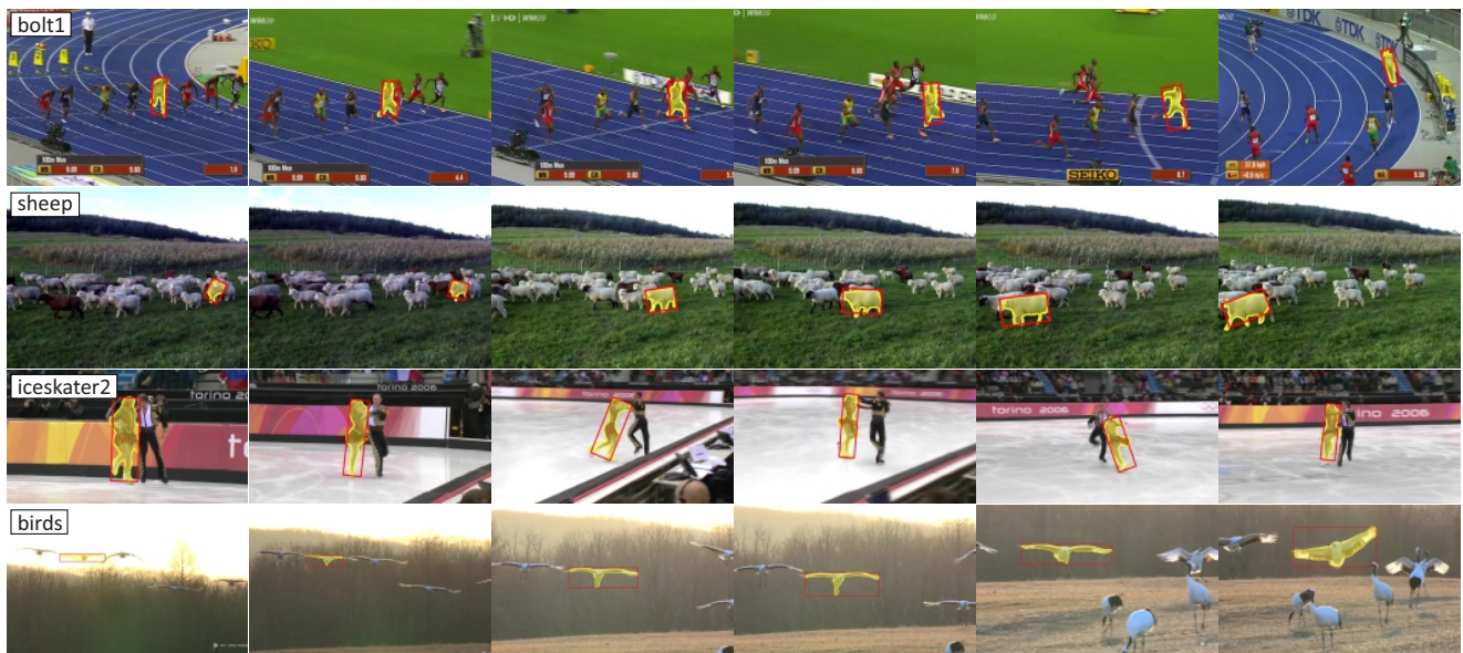
Figure 1. Sequences with distractors (similar objects in the target vicinity). D3S segments the correct target even though a similar target is close (or even overlapping). These examples show discriminative power of the proposed tracker achieved by the discriminative GIM and GEM.
