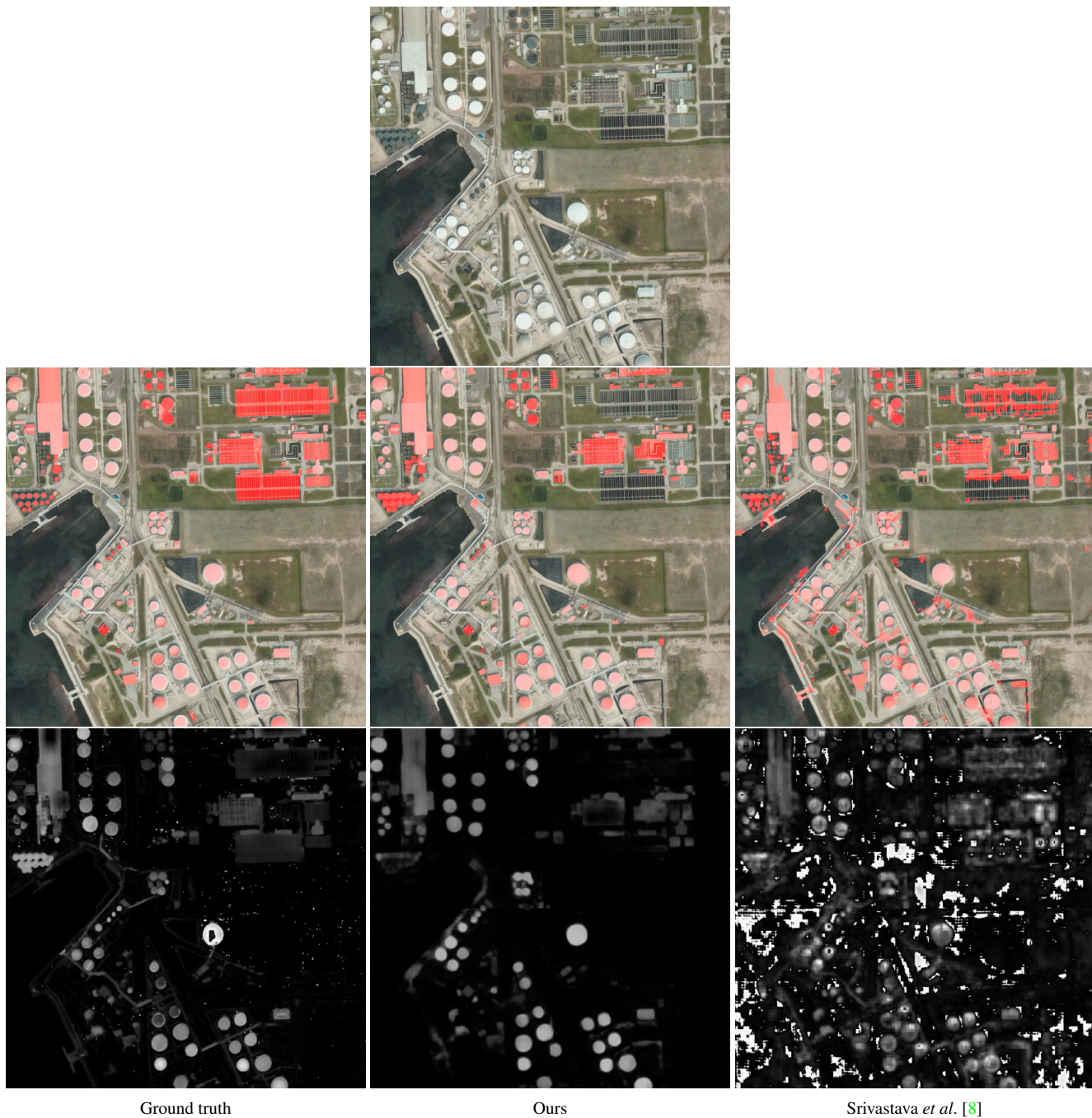
Figure 12: Additional results on the Urban3D dataset for our method versus [8]. First row: aerial image. Second row: predicted building instances overlaid on the overhead image. Third row: nDSM. Our prediction apparently does not capture two ground-truth building instances in the top-right corner. However, the ground truth may be incorrect for both of these instances, as we can observe roads passing through them. When visualized in Google Earth, as well, these instances do not appear to be buildings.
