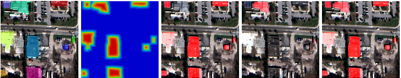
Figure 1: From left: Overlapping proposals from Task 1, predicted BPSH, building masks after NMS, additionally recovered building proposals, and final building masks. The overlapping proposals are the purple and teal buildings in the top left, where the teal proposal actually covers two buildings, and the purple proposal overlaps the part of the teal that covers the smaller building.
