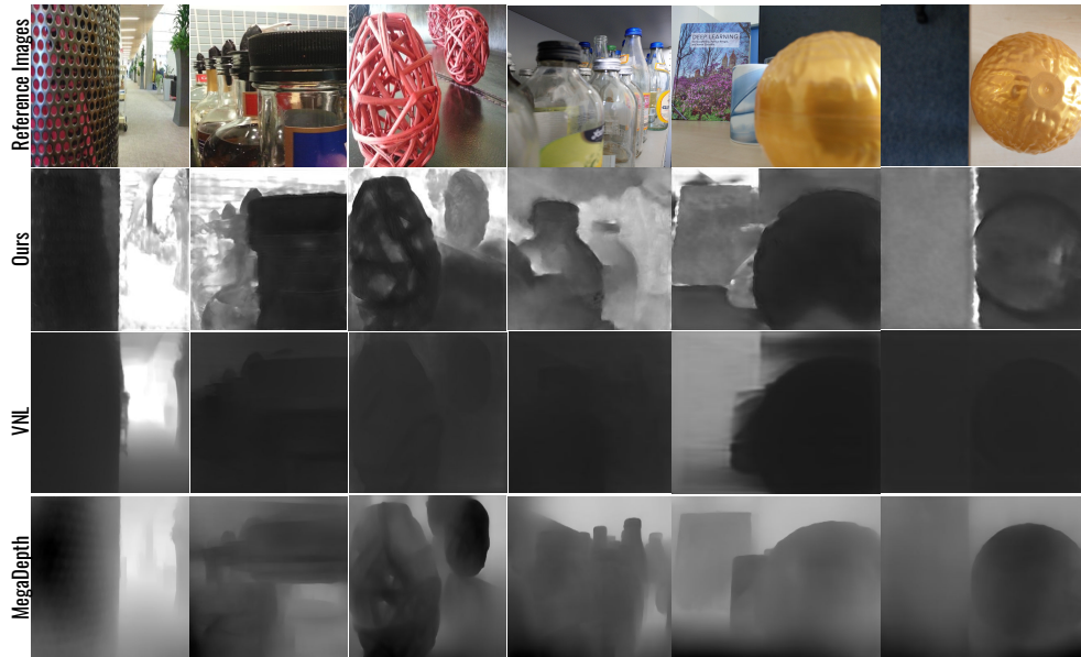
Figure 5: Depth estimation comparison on real data. 1st row: input images, 2nd row: our results on a focal stacks (with 2 images) , 3rd row: results of VNL [9], 4th row: results of Megadepth [5] - on single images. First 3 images are from MobileDepth [8] dataset and next 3 images are taken with a smartphone.
