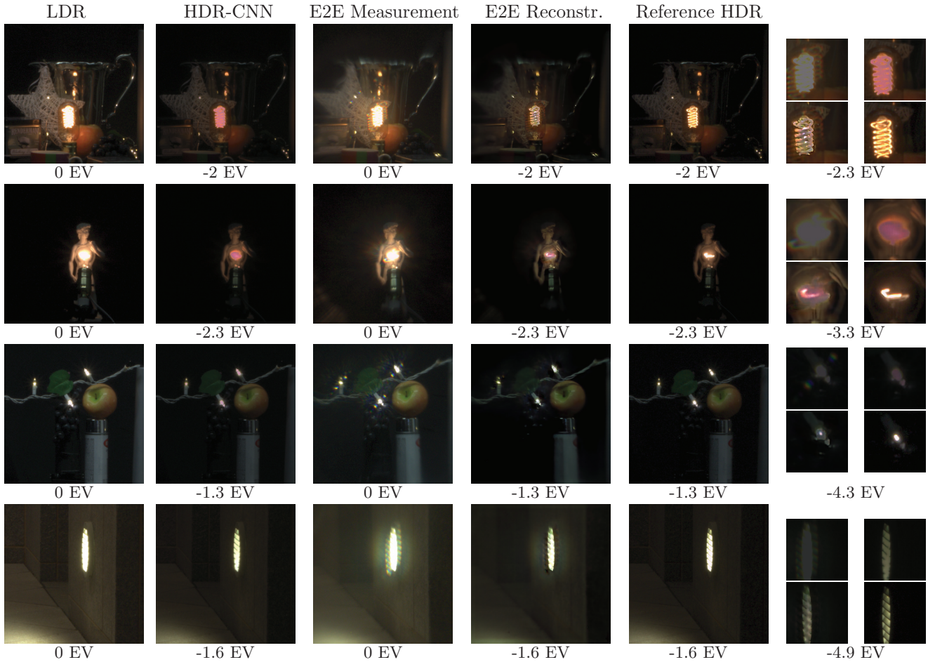
Figure 2: Experimental data of three indoor scenes (top three rows) and one outdoor scene at night (bottom row). The limited dynamic range of the sensor loses details in the brighter parts of the captured LDR image (first column) as compared with the reference HDR image (fifth column). A CNN operating directly on the LDR images hallucinates brighter content in these saturated parts, but it is missing the detail (second column). The measurements captured with our prototype camera optically encode this detail in the image by superimposing several scaled and shifted copies of the image on itself (third column). This information is used by our CNN to recover the missing parts of the scene while digitally removing the image copies (fourth column). The closeups show that deep optics is more successful in recovering bright detail of HDR scenes than other single-shot HDR imaging approaches (right column).
