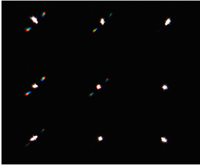
Figure 3: Image of nine point sources from different regions in the camera's field of view (FoV). To deal with the spatially variant PSF, we crop the FoV to the center and train our network on the PSF there.
