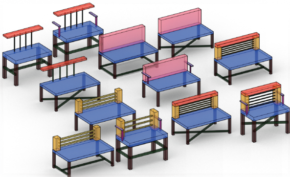
Figure 2. Synthetic chair variations. We show a few examples of the 96 structural variations of a bench, including variations to the legs, base, backrest, and armrests.
