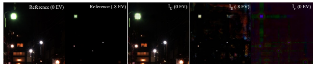
Figure 5. Intermediate images of our network for the first scene in Fig. 4 of the paper. \hat{I}_U shows that the streak encodings have been correctly removed. \hat{I}_S is displayed at -8 EV and shows accurate reconstruction of highlights. The residual image \hat{I}_r shows that the streaks have been identified and separated from the input image.
