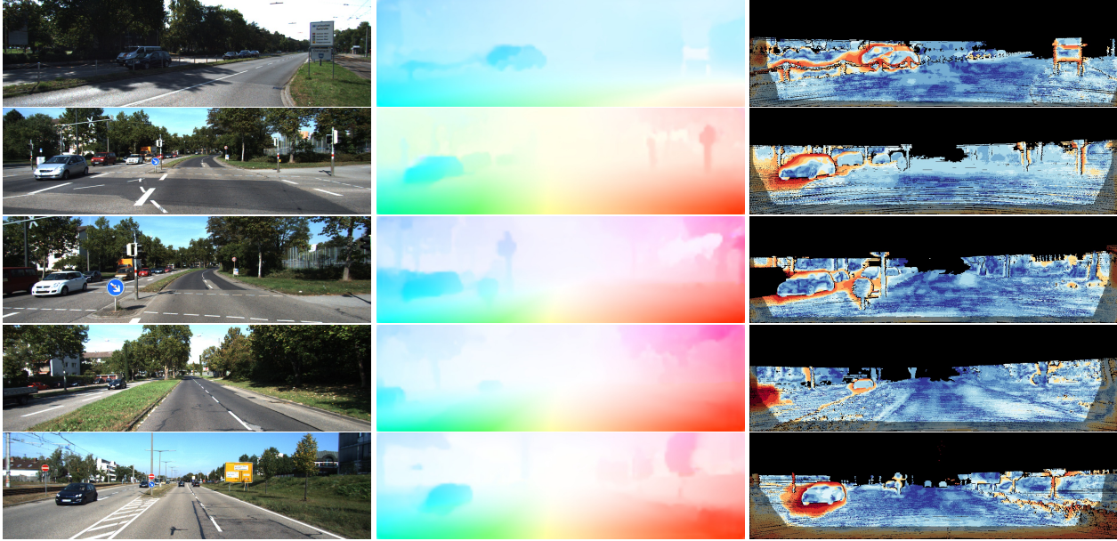
Figure 6. Visualization of the flow error map of our optical flow network on the KITTI 2015 testing benchmark. Larger errors are encoded in red, while blue pixels represents good optical flow estimates with respect to the ground-truth.
