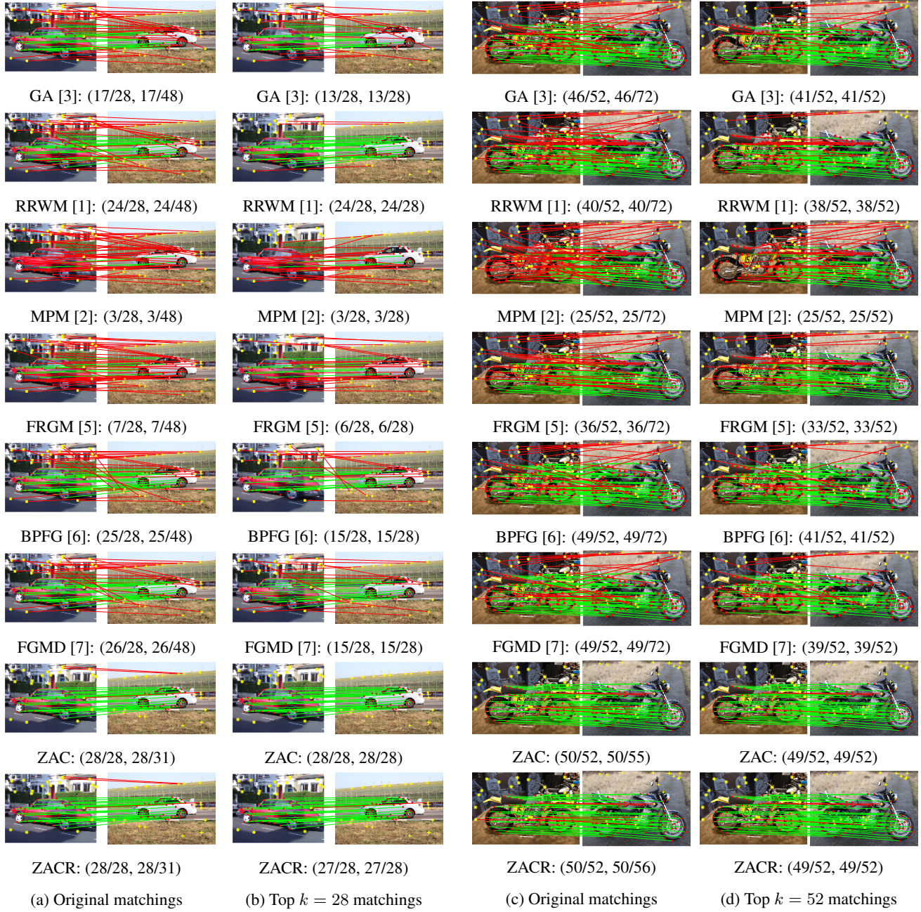
Figure 3: Examples of graph matching with inliers (red dots) and outliers (yellow signs) on the car images (left two columns) and motorbike images (right two columns) in PASCAL dataset. For each method, the recall and precision are computed with their original matchings and top k = \#inliers matchings, respectively.
