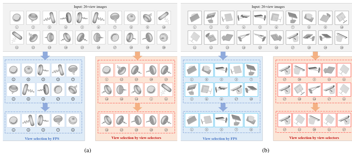
Figure 4. Illustration of selected views for constructing hierarchical view-graphs by FPS and our view-selector. (a) View selection by FPS (blue) and our view-selector (orange) for an object of flower pot. (b) View selection by FPS (blue) and our view selector (orange) for an object of monitor. For different shapes, our view selector can sample the views adaptively, while FPS takes fixed views. The input objects are with 20 views, and coarsened twice to 10 and 5 views to build coarsened view-graphs. Our sampled views using view-selectors produce better results as discussed in experiments.
