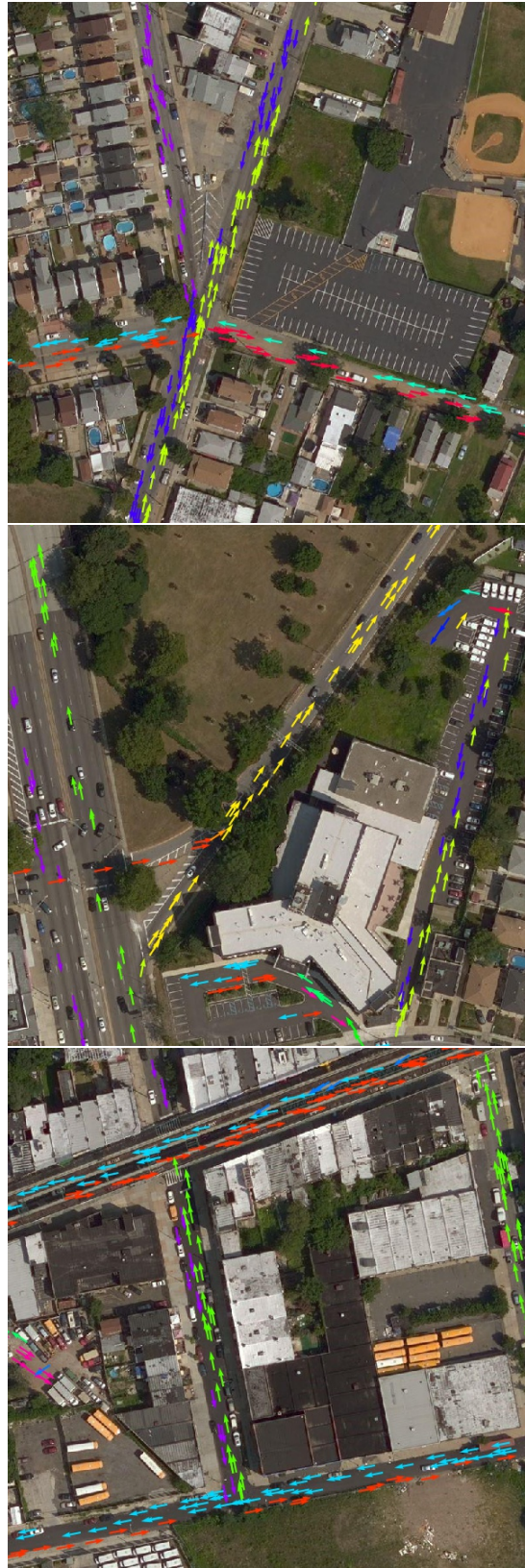
Figure 8: Using our approach to estimate directions of travel (visualized as flow fields).
