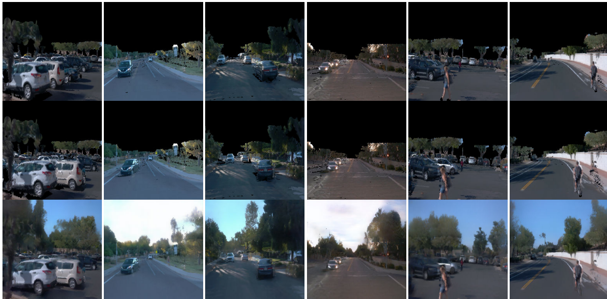
Figure 10. Synthesized images by perturbing objects in the scene. Top row: original surfel rendering. Center row: surfel rendering after perturbing the objects. Third row: synthesized images.
