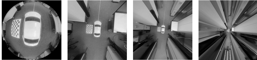
Fig. 2. De-warping of a FE image: Left to right: original FE image and rectilinear de-warped images with decreasing focal length of the virtual camera. By increasing the focal length of the virtual camera, the field of view decreases and information content from the FE image is lost.
