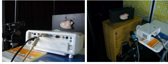
Fig. 9. Actual objects capturing setup. A camera and a projector are precisely calibrated in advance.
