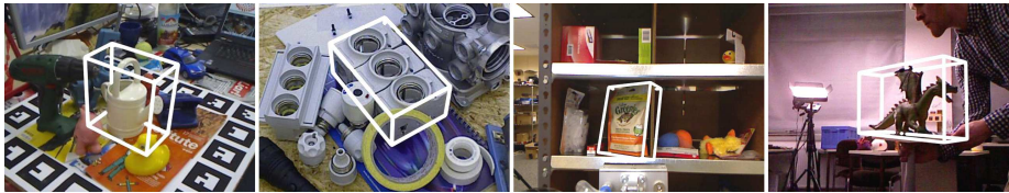
Fig. 1. Estimation of 6D pose, i.e. 3D translation and 3D rotation, of a specific rigid object. This task is considered in the BOP benchmark [25].
