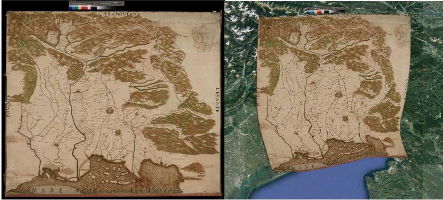
**Fig. 1.** Example of an historical map georeferencing process. Left: original map (1682, Sebastiano Alberti, ASV). Right: georeferenced map with respect to 15 manually defined control points overlapped to a satellite view of the area (Google Earth basemap). Map image courtesy of State Archive of Venice.
