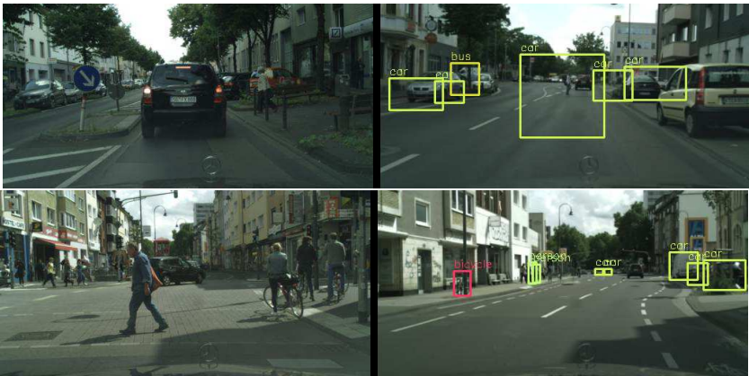
Fig. 4: Examples of street scene object forecast. Left column shows current frames, while right column shows frames after 1.8 seconds.
