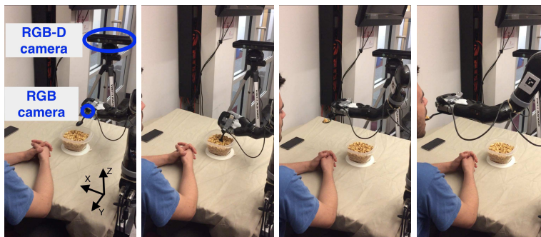
Fig. 1: Our feeding system includes a MICO robot arm, an RGB-D camera, and an RGB camera. The first image also labels the axis orientations of the robot coordinate system.
