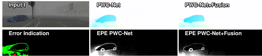
Fig. 3: Visual results of our fusion method. Green in the indication map means that PWC-Net+Fusion is more accurate than PWC-Net, and red means the opposite.
