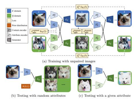
Fig. 3: **Method overview.** (a) With the proposed content adversarial loss  $L_{\rm adv}^{\rm content}$  (Section 3.1) and the cross-cycle consistency loss  $L_{\rm 1}^{\rm cc}$  (Section 3.2), we are able to learn the multimodal mapping between the domain  $\mathcal{X}$  and  $\mathcal{Y}$  with unpaired data. Thanks to the proposed disentangled representation, we can generate output images conditioned on either (b) random attributes or (c) a given attribute at test time.
