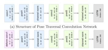
(b) Structure of Deformable Pose Traversal Convolution Network
