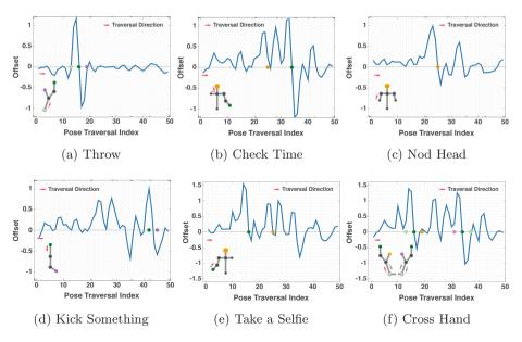
Fig. 7: Visualization of the Learned Offsets. The blue curve shows the offset for convolution kernel on each anchor. The sketch on the corner of each sub-figure shows the part of the pose that has high offset response in offset learning. The colors of the joints in the sketch correspond to the colored marker on the x-axis of the figures. The red arrows in the sketch guide the direction of the traversal.
