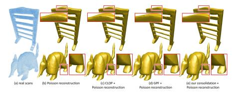
Fig. 7: Comparing reconstruction results on real scans produced by direct reconstruction (b) and with consolidation: CLOP, GPF, and our method (c-e).
