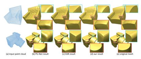
**Fig. 6:** Comparing surface reconstruction results produced by using PU-Net (b), EAR (c), and our method (d) to consolidate points with the original meshes (e).
