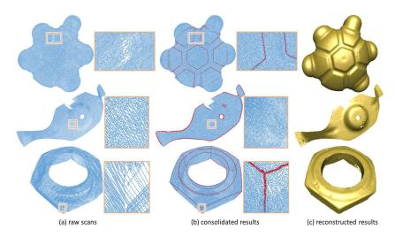
Fig. 9: Three results from real scans (a). Note the diversity of the geometry, the sparseness of the inputs (a), and how well the network locates the edges (in red); see (b). The reconstruction results (c) are yet imperfect due to tiny regions that are severely undersampled (see the blown-up views in (a)).
