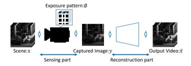
**Fig. 1. Compressive video sensing.** A process of encoding multiple sub-frames into a single frame with controlled sensor exposures, and reconstructing the sub-frames from a single compressed frame.
