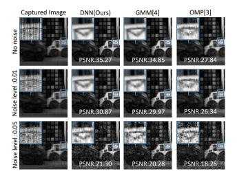
Fig. 10. Reconstruction results of 3rd sub-frame with different noise levels by the deep neural network (DNN), Gaussian mixture models (GMM), and orthogonal matching pursuit (OMP) (exposure pattern: optimized RCE)
