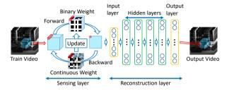
**Fig. 5. Network Structure.** Proposed network structure to jointly optimize the exposure pattern of compressive video sensing, and the reconstruction. The left side represents the sensing layer that compresses video to an image by using the exposure pattern. The right side represents the reconstruction layer that learns non-linear mapping between the compressed image to video reconstruction.
