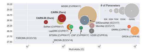
Fig. 4: Trade-off between performance vs. number of operations and parameters on Set14  $\times 4$  dataset. The x-axis and the y-axis denote the Multi-Adds and PSNR, and the size of the circle represents the number of parameters. The Mult-Adds is computed by assuming that the resolution of HR image is 720p.
