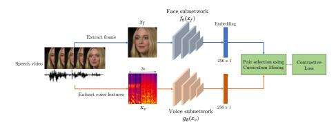
Fig. 1. Learning a joint embedding between faces and voices. Positive face-voice pairs are extracted from speech videos and fed into a two-stream architecture with a face subnetwork  $f_{\theta}(x_f)$  and a voice subnetwork  $g_{\phi}(x_v)$ , each producing 256-D embeddings. A curriculum-based mining schedule is used to select appropriate negative pairs which are then trained using a contrastive loss.
