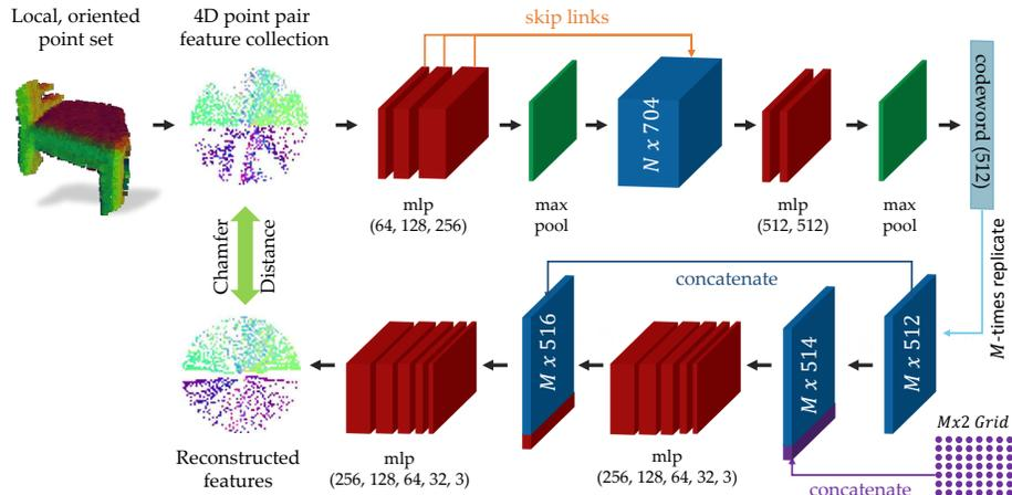
**Fig. 1.** PPF-FoldNet: The point pair feature folding network. The point cloud local patches are first converted into PPF representations, and then sent into the encoder to get compressed codewords. The decoder tries to reconstruct full PPFs from these codewords by folding. This forces the codewords to keep the most critical and discriminative information. The learned codewords are proven to be robust and effective as we will show across extensive evaluations.
