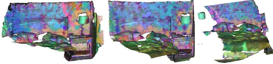
**Fig. 7.** Visualization of the latent feature space on fragments fused from different views. To map each feature to a color on the fragment, we use TSNE embedding [24]. We reduce the dimension to three and associate each low dimensional vector with an RGB color.
