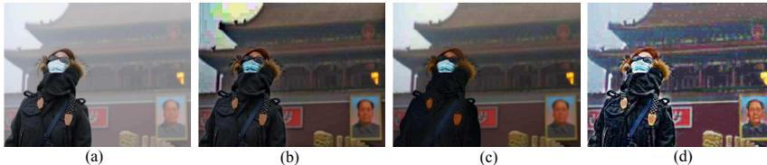
**Fig. 1.** An illustration of image dehazing. (a) A hazy image. (b), (c) and (d) are the images after applying different dehazing methods to the image (a).
