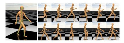
Fig. 3. Left: The humanoid model. Green arrows illustrate 3D vectors from the root to the feet, head and hands provided to the policy and discriminator. **Right:** Selected key frames of running and walking clips in motion capture data animated using the humanoid model.
