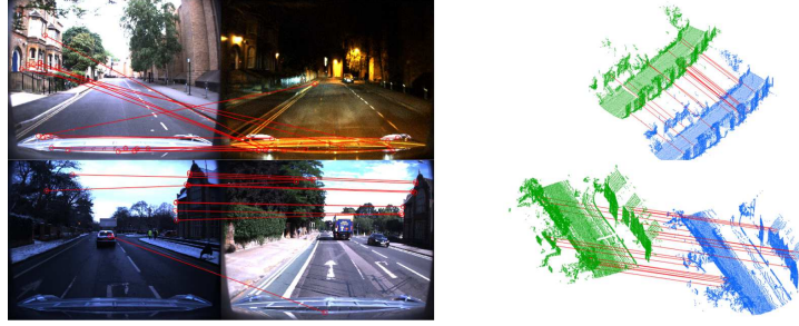
Fig. 1. Left: 2D images from the Oxford dataset at different times of the day (top) or seasons of the year (bottom) give mostly wrong matches even after RANSAC. Right: 3D point cloud of the same scene remains largely the same and can be matched easily.
