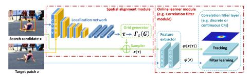
Fig. 2: Pipeline of our algorithm. Note that the red bounding box in the search patch  $\mathbf{x}$  represents the initial candidate target position and the yellow one represents the aligned position provided by our SAM. Our SAM is generic and the CF module can be replaced by other online tracking learners.
