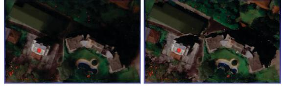
Figure 11: Weighted average of the colour information with and without the shadowed areas. Note how much information is recovered on the right when using only lit images.
