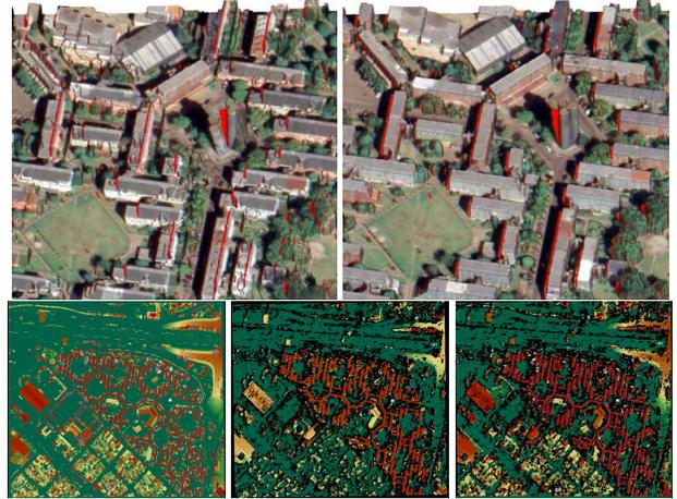
Figure 8: Top: Projection on the mesh obtained from the Lidar of image  $I$  before and after the registration step. Bottom: Lidar, DSM from S2P associated with image  $I$  before and after registration, all represented with the same colormap. The translation vector obtained from gradient correlation is  $T_A = (-6.94985 \text{ pix}, -20.2493 \text{ pix}, -3.06814 \text{ m})$ .
