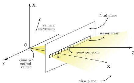
Figure 2: Linear push-broom camera model. The instantaneous camera optical centre  $C$  moves at a constant speed. The view plane sweeps out the whole 3-space as the camera moves forward. The 3D point  $X$  is imaged by the camera to the focal plane location  $x$  [6, 20].
