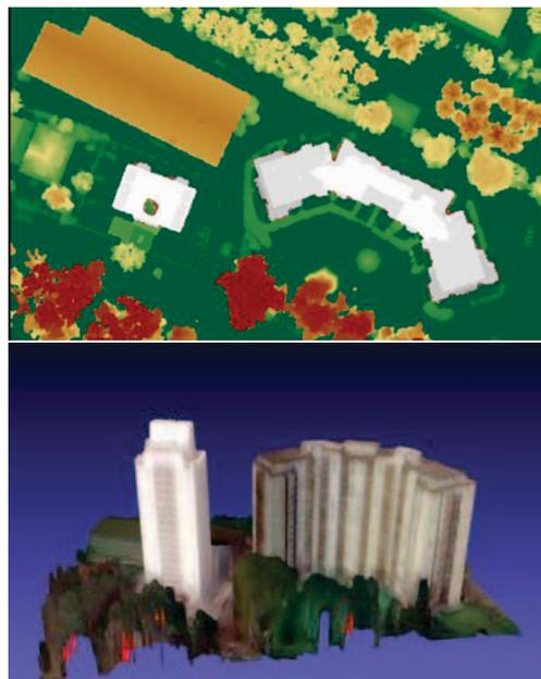
Figure 1: Top: detail of the Lidar provided in the IARPA dataset. Bottom: textured mesh obtained using the Lidar and the 47 satellite images of the dataset. The texturation adds a new dimension and allows a better understanding of the reconstructed area.
