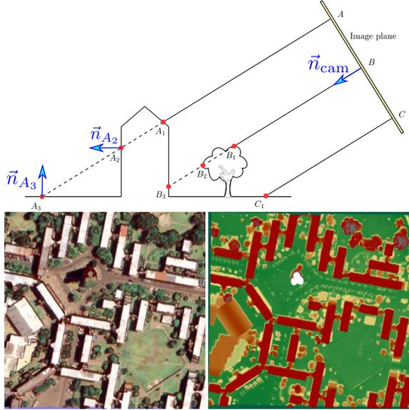
Figure 9: Top: sketch of the projection of the mesh onto the image plane. Bottom left: mesh textured from one image, seen from the camera viewpoint. Bottom right: elevation of each point seen by the camera on the image plane.
