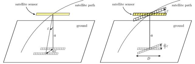
Figure 5: Effect of attitude errors on the localisation function. The figure on the left shows a pitch error of  $\epsilon$ . To first order, this induces a ground displacement of the sensor projection of  $a\epsilon$ , where  $a$  is the flying altitude of the sensor. The figure on the right shows a yaw error of  $\epsilon$ . It induces a maximal ground displacement of  $\frac{D}{2}\epsilon$ , obtained for the sensor endpoints, where  $D$  denotes the swath width [6].
