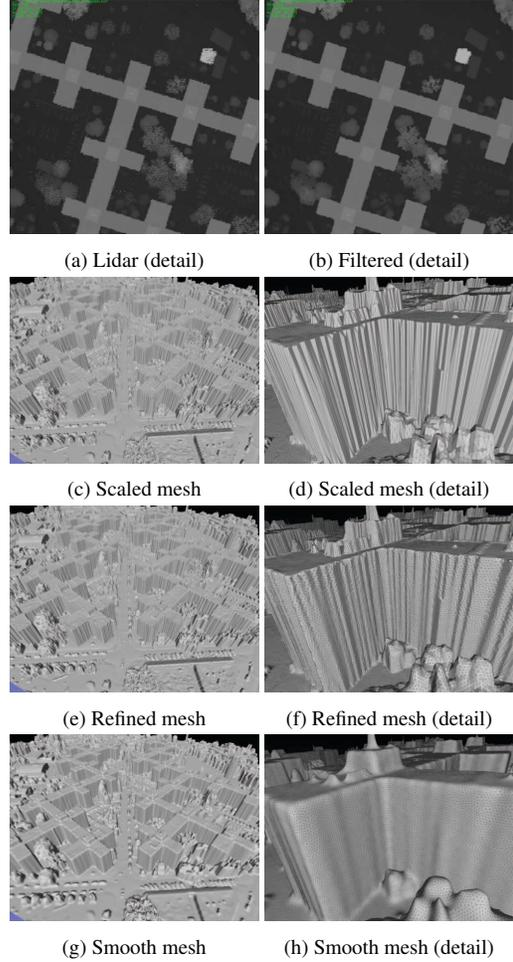
Figure 7: Steps described in Subsection 3.1 for the creation of a smooth mesh from a reference DSM.
