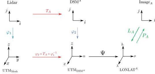
Figure 6: This figure illustrates all the coordinates system we use for the pipeline. The localisation and projection functions,  $L^A$  and  $P^A$ , are found in the metadata of the satellite image  $A$ . The functions  $\varphi_1$  and  $\varphi_2$  are the inverses of the functions used to project the georeferenced point clouds onto the DSMs. The vector  $T_A$  corresponds to the geolocation error.  $\Psi$  translates UTM coordinates into longitude-latitude.
