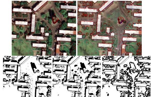
Figure 10: Top: image projected on the mesh before and after a shadow removal step [5]. Bottom: predicted shadow from geometry, shadow from thresholding and estimated shadow boundary.
