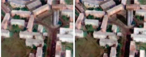
Figure 14: Left: mesh textured after a shadow-less osmosis-based fusion performed with  $f = F_{2,3}$ . Right: same result after adding back shadows. Note how it makes the tower and the trees easier to distinguish.
