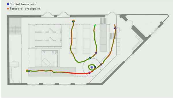
Figure 8: Trajectory performed by a test user projected on the gym map showing: speed changes, spatial breakpoints and temporal breakpoints.
