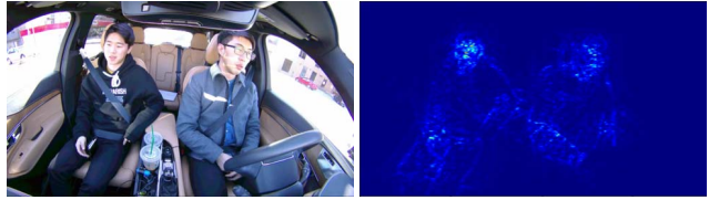
Figure 6: Saliency map visualization [31] for the ‘right wrist’ class. Note visual cues from the face have significant contribution to the prediction.
