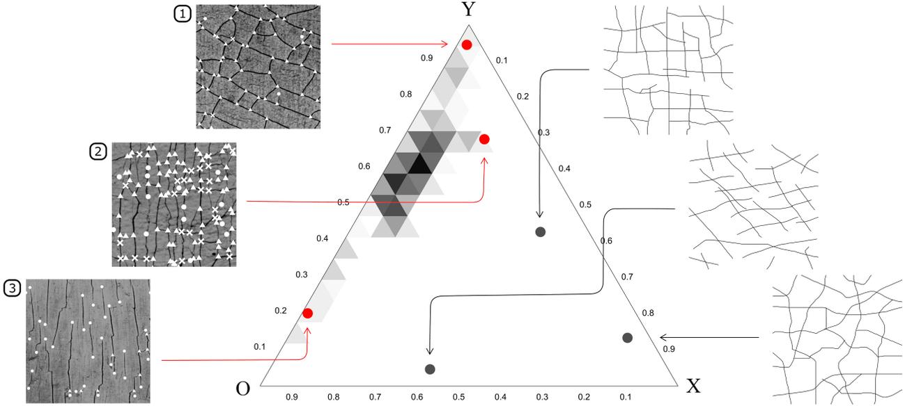
Figure 2. Triangular topography chart. Each point is defined by three coordinates  $(N_O, N_Y, N_X)$ . Darkened areas illustrate distribution of natural craquelure network on the chart (darker color - higher density). Real samples shown: (1) - XVI century Flemish panel; (2) - Jan van de Cappelle, "River scene with a large ferry", canvas painting, 1665; (3) - Duccio, "The Annunciation", panel, 1307/8.
