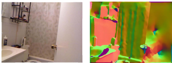
Figure 4: A common example of the errors seen in the normals from [16] that many use for training and evaluation. In these visualizations, (r, g, b) map to (x, y, z) of the normal at that location. Note the oversmoothing, which reduces and removes the normals of small objects. This image also demonstrates why it is important to only backpropagate on pixels that have valid depth, as the right side of the image has incorrect normal data due to noisy and missing depth values.
