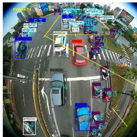
Figure 13. Fisheye lens-based traffic analysis system.
