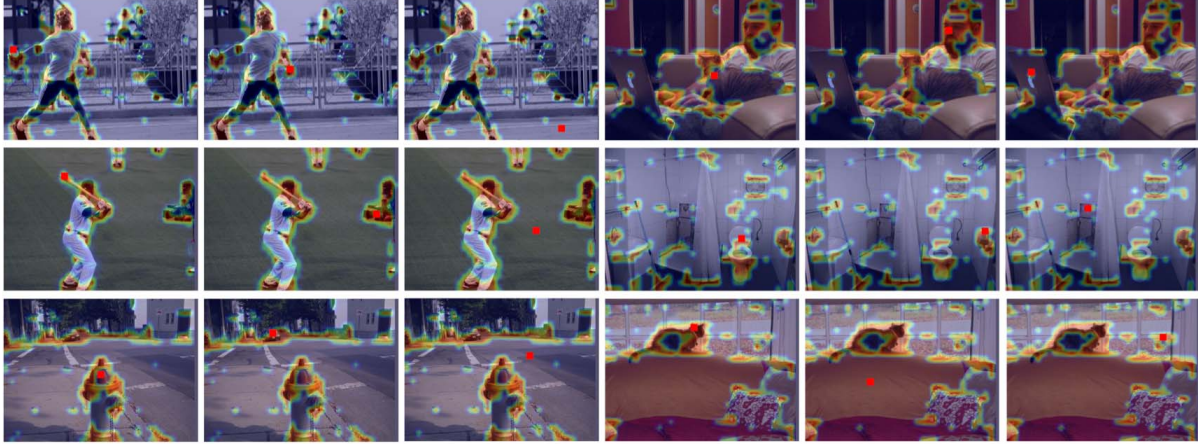
Figure 2: Visualization of attention maps (heatmaps) for different query positions (red points) in a non-local block on COCO object detection. In the same image, the attention maps of different query points are almost the same. Best viewed in color.
