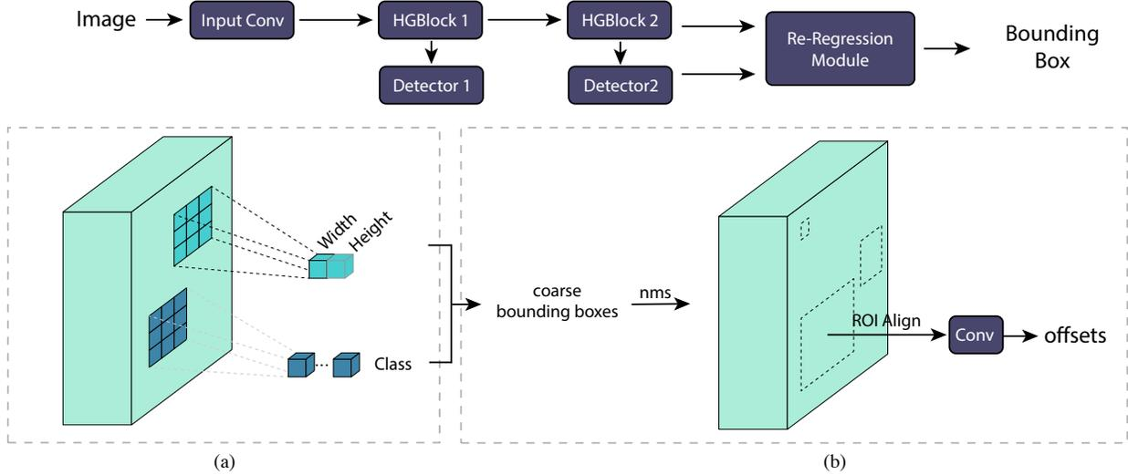
Figure 5. The architecture of the RRNet. (a) The detector in the RRNet. We only present the prediction for one feature pixel. We perform the same prediction on all the feature pixel. (b) The Re-Regression Module.
