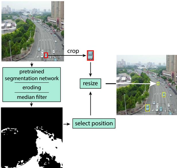
Figure 3. The pipeline of AdaResampling.
