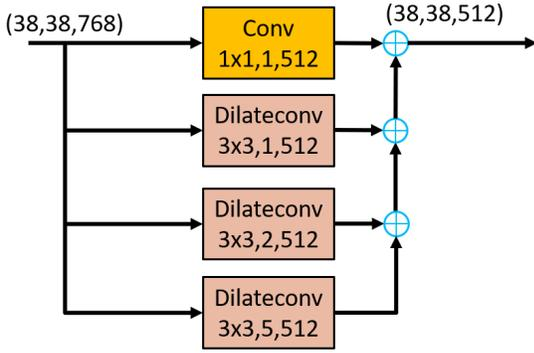
Figure 4. Feature Decomposition Module architecture.
