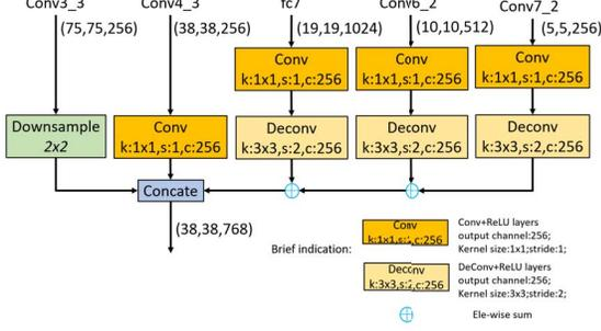
Figure 3. Feature Fusion Module architecture.
