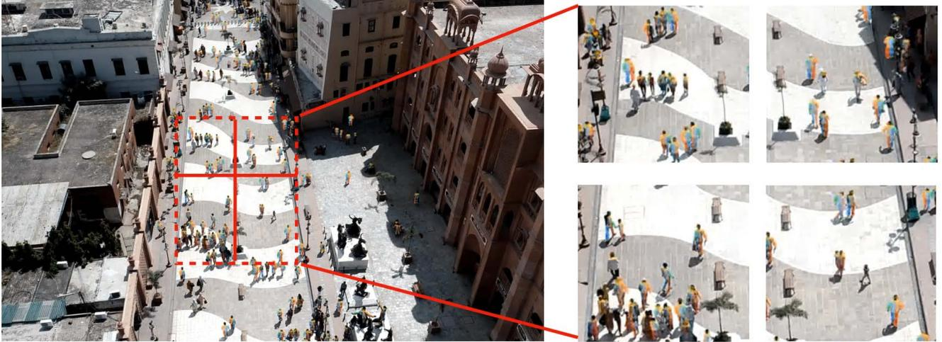
Figure 4. Human Detection at different Scales: Pose estimation is performed for humans which appear at different scales by dividing the 4K resolution frames recorded by the UAV into 72 regions as shown. Selected regions are shown. The reasoning for this processing is detailed in section 3.1.
