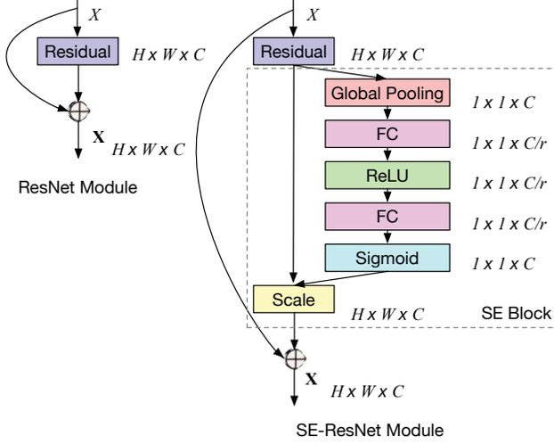
Figure 6. The structures of ResNet and SE-ResNet modules.
