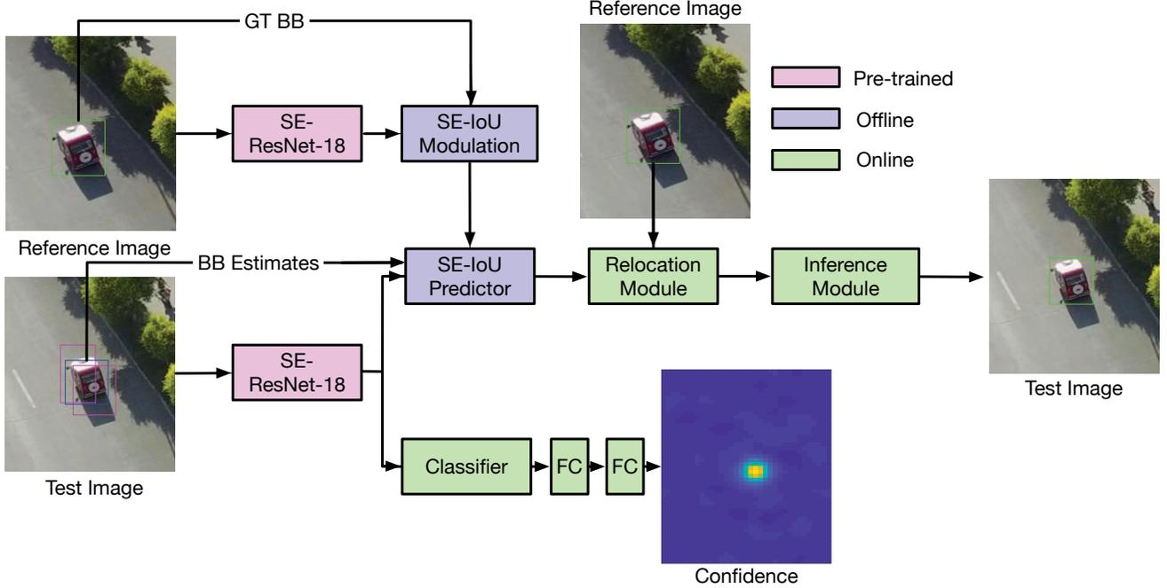
Figure 5. The framework of the proposed tracker ATOMFR (RL + InF).
