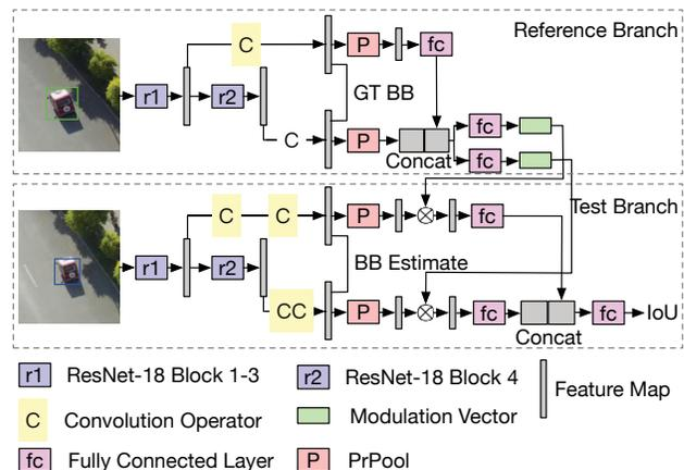
Figure 4. The framework of the target estimation network in ATOM.
