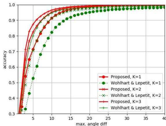
Figure 6. Pose recognition accuracy for different levels of maximum accepted pose difference.  $K$  denotes the number of nearest neighbours. The proposed method significantly outperforms the state of the art RGBD deep pose descriptor.
