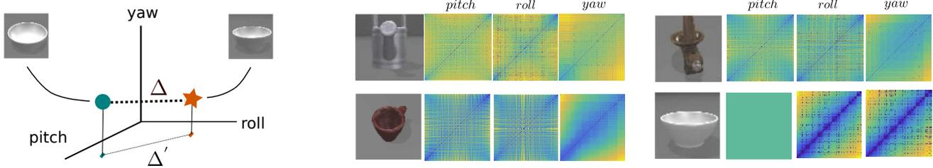
Figure 2. (left) Illustration of the case of  $s_{yaw} = 0$  for a simple case of a fully rotationally invariant object for the yaw axis. (right) Illustration of the  $\phi$  term (Equation 5) for all pose pairs individually per 3D axis. Note that the more symmetric objects present lower values than the non-symmetric ones.
