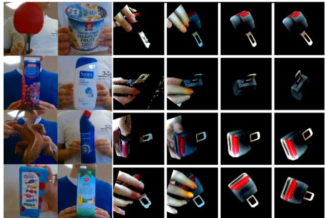
Figure 9. (left) Objects from our real captured occlusion dataset (right) Results for the tracker-based occluded dataset. 1<sup>st</sup> column shows a real RGBD image, 2<sup>nd</sup> shows the image rendered using the tracking annotation, 3<sup>rd</sup> shows the rendered object corresponding to the occluded image, 4<sup>th</sup> shows the nearest neighbour retrieved using our pose-guided features.
