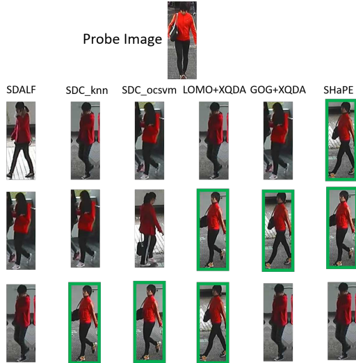
Figure 3: A person re-identification example showing top 3 matches for a sample probe image from CUHK01 dataset. Correct matches are shown in a green bounding box.
