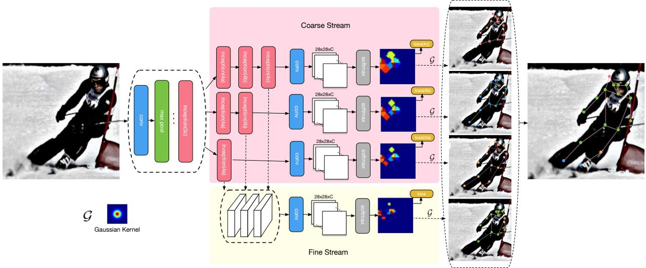
Figure 2: The network architecture of CFN. The coarse stream learns three coarse keypoint detectors using multi-level supervisions and while the fine stream learns a fine detector via strict supervision. Then the coarse predictions and fine predictions are unified for final prediction at the inference stage.
