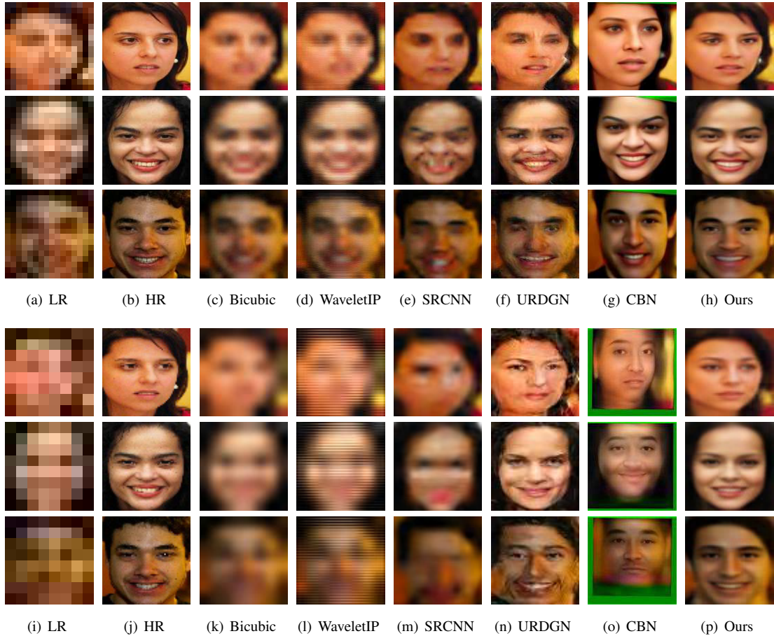
Figure 5. Comparison with state-of-the-art methods on very low input resolutions. The input resolutions are 16 \times 16 and 8 \times 8 for the top three and bottom three rows, respectively. The magnifications are both 8\times . Images are selected randomly from Helen test set. We do not try to crop the green area caused by the shape transform of CBN in (g) and (o) to avoid facial deformation.
