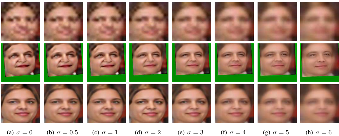
Figure 6. Robustness toward unknown gaussian blur on Helen test set. The input resolution is 16 \times 16 and the magnification is 8\times . The top, middle and bottom rows are the results of bicubic interpolation, CBN and ours, respectively.
