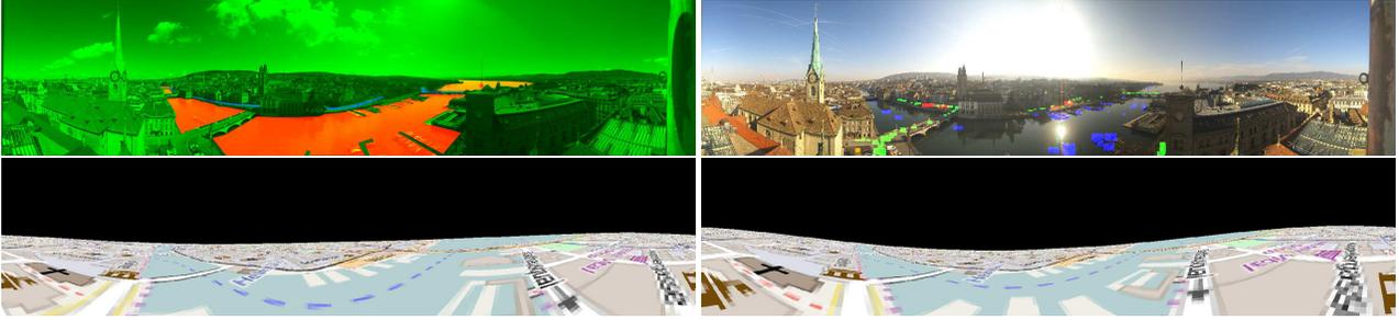
Figure 3: Top left: Segmented regions (river in red and tramway in blue) selected manually; top right: automatically detected objects (boats in blue, trams in red, and cars in green) from an image sequence recorded over a day. An example of the warped map (on the image) obtained using our method before (bottom left) and after (bottom right) the refinement step.
